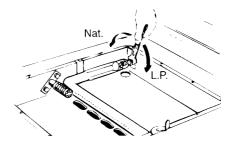
To shorten the cones, tighten the orifice hood by turning in the "LP" direction. To lengthen the cones, loosen the orifice hood by turning in the "Nat." direction.
